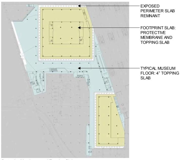
Footprint Slab: Protective Membrane and Topping Slab
